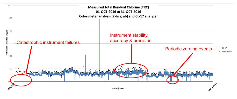
Cl-17 and colorimeter TRC values were paired at the grab sample time and tested for statistical relevance.
